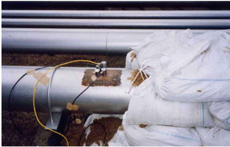
Fig. 5 AE sensors mounted on a simulated buried pipe.
