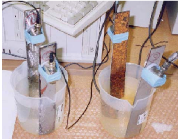
Fig. 2 Four specimens in 3% salt water (Test 1).
