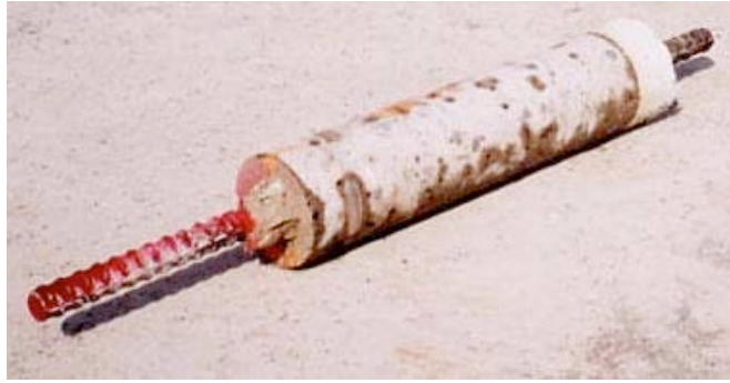
Fig. 3 A cored sample including a steel bar.
